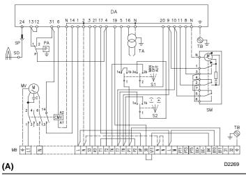
**Factory Wiring Diagram** RS 38/M - RS 50/M three-phase With Siemens LFL control
